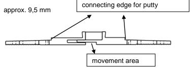
**Application:** for expansion joints in ceramic, textile and elastic floor coverings
